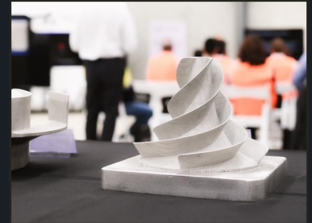
Hydro pulper printed in 316 stainless steel
