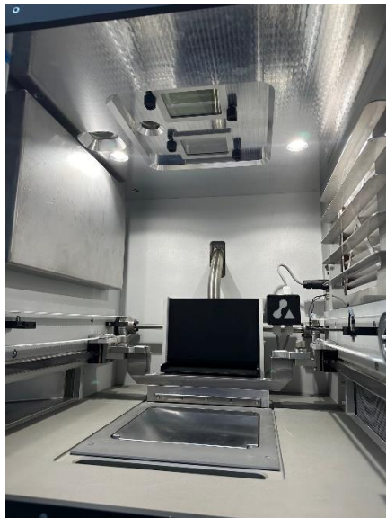
The chamber is prepared for printing in the AL250 as it goes through final calibration steps.
