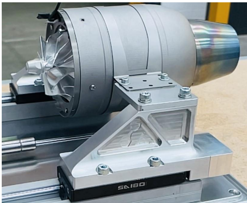
Figure 2: 3D Printed gas turbine, being readied for inspection after successful test fire.
