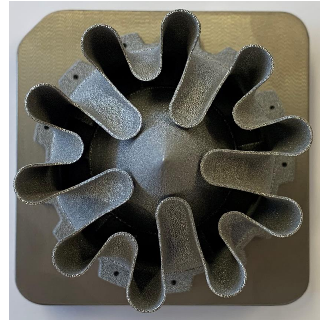
Turbine fuel mixer printed on Alpha RMT printer
