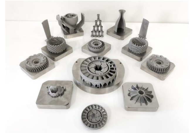
All parts printed on Alpha RMT printer
