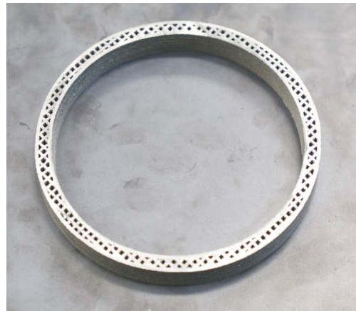
Ring with mass reducing hatch in NiSiB
