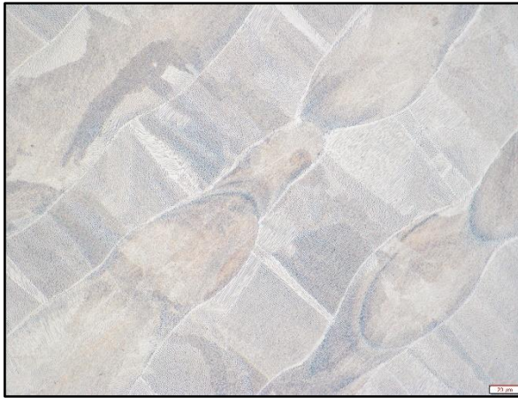
Metallographic samples at 200 x magnification following etching with electrolytic 10% Oxalic acid
