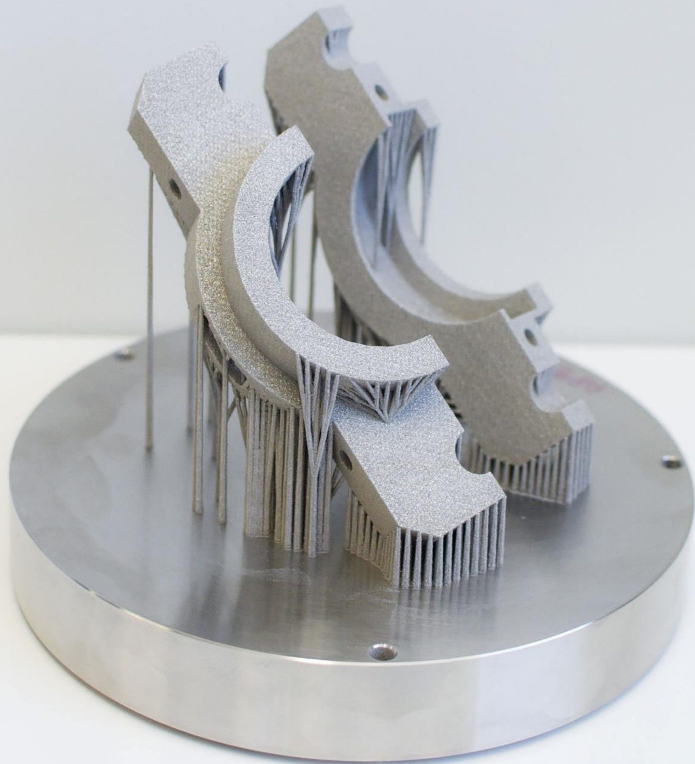
Gland Follower 3D printed by Aurora Labs. A common component in many pumping systems.
