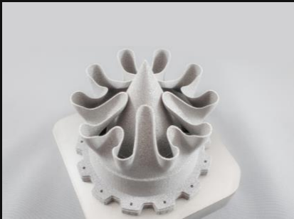
Turbofan exhaust mixer printed on Alpha RMT printer
