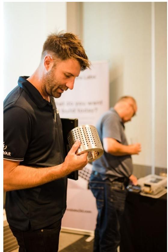
Figure 2: A3D printed stainless steel valve trim
